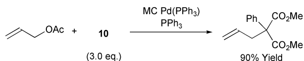
Scheme 19 Allylic substitution of allyl acetate with 10 . Reagents and conditions: MC Pd(PPh 3 ) (20 mol%), PPh 3 (20 mol%) BSA (3.0 equiv.), KOAc (0.10 equiv.), CH 3 CN, reflux, 12 h.
